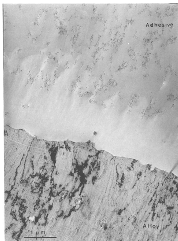
Figure 15 Interface adjacent to crack tip in a specimen with an etched aluminium surface.
